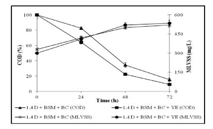
Fig. 5: COD and MLVSS profile during 1,4 dioxane biodegradation in the presence of Yeast Extract
