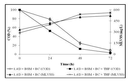
Fig. 6: COD and MLVSS profile during 1,4 dioxane biodegradation in the presence of THF
