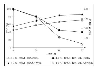
Fig. 4: COD and MLVSS profile during 1,4 dioxane biodegradation in the presence of Glucose
