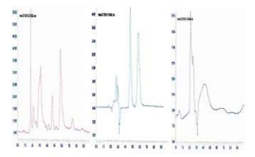
Fig. 5: HPLC Chromatogram a) Showing Atrazine concentration more than Simazine. b) Showing Simazine concentration more than Atrazine. c) Showing no peak in the interested area
