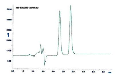
Fig. 4: HPLC Chromatogram obtained by analyzing Spiked water Sample
