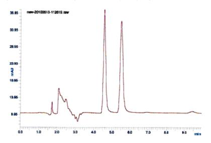
Fig. 3: HPLC Chromatogram obtained by analyzing Standard Simazine & Atrazine
